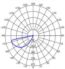
Beam Angle(50%) C0-180,C90-270: 330.0 deg,157.3 deg
